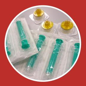
The proposed technology is able to **sterilize bulk or pre-oackaged items**, through the indirect action of a **non-thermal plasma**. The invention claims to be an alternative to other existing methods of sterilization, e.g. usig ethylene oxide (EtO).
