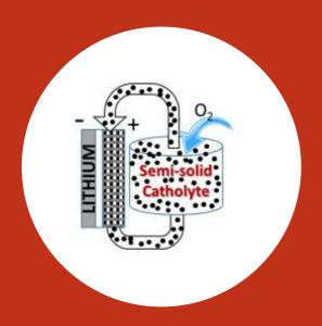
Lithium/oxygen non-aqueous semi-solid flow battery that combines the high energy density of lithium/air batteries with the flexibility of redox flow batteries.
