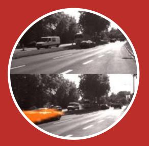
Method for estimating depth, optical flow, and other semantic information on low-power devices. Specifically, low-resolution images acquired from a single camera are processed by a lightweight and highly accurate selfsupervised Convolutional Neural Network.
