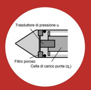
The invention includes the method and apparatus necessary to establish a quantitative criterion defining the saturation degree of the sensor group in a piezocone tip.
