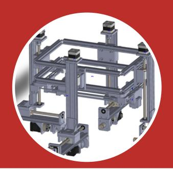
Mobile 3D printer for manufacturing tubular objects of variable cross-section without length constraint, and capable to move and print along the object without any external support. The system's capabilities are enabled by the mobility component coupled with a gripping system integrated into the object.
